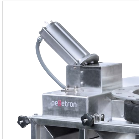
DeDuster® models XP180 to XP1500 can be equipped with an automated inlet deflector to distribute the material evenly over both wash decks. This option eliminates the need for the installation of a separate feeding device
